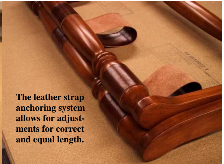
A leather strap attached to a spindle in the completed stand. Note the small brown felt pad on the curve of the leg to protect the stand when it is folded.
